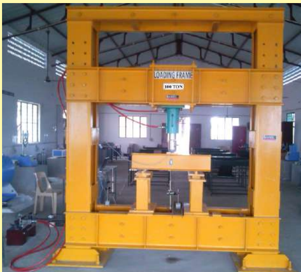
Computerized Load Frame
