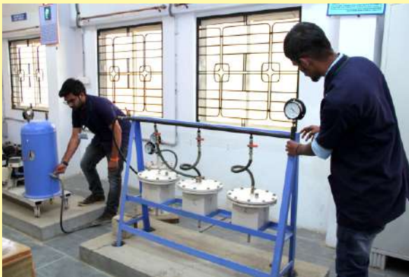
Concrete Permeability Apparatus
